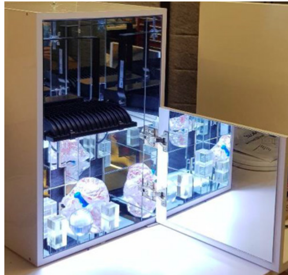
Figure 7: Sample do-it-yourself photobleaching cabinet with LED lamp and mirrors.
