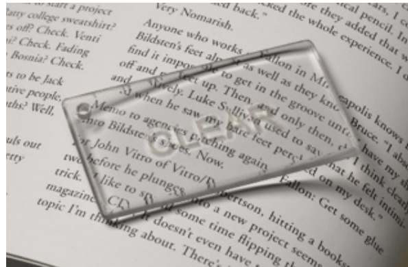
Figure 5: Polished and lacquered part, printed with VeroClear.
