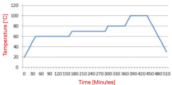
Figure 9: Oven temperature over time (Procedure B).
