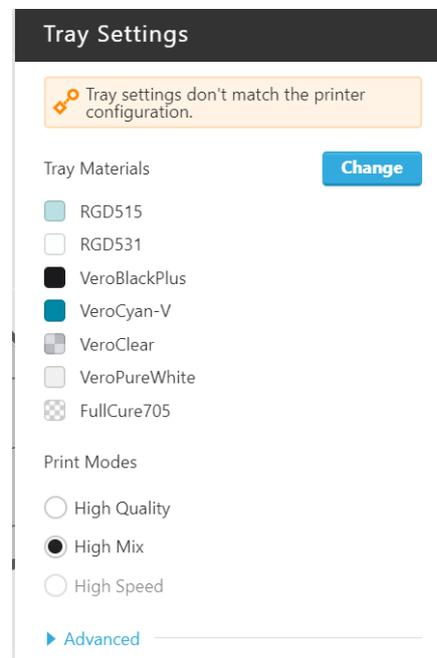
Figure 2: Digital ABS material selection in GrabCAD Print™.
